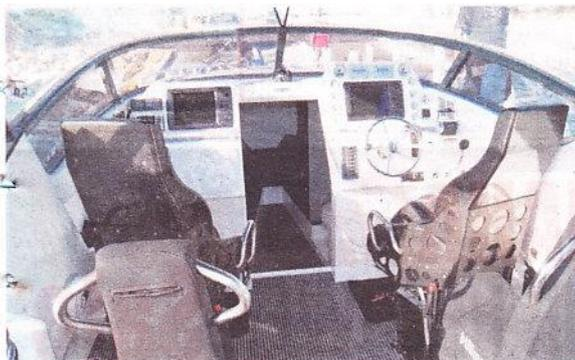
The neatly set out dash houses a pair of 12-inch screens for a Raymarine package of 3-D sounder, GPS and radar.
